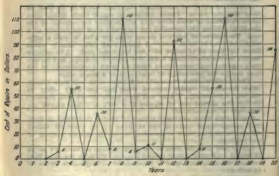
Fig. 1. Repairs of Freight Car.
